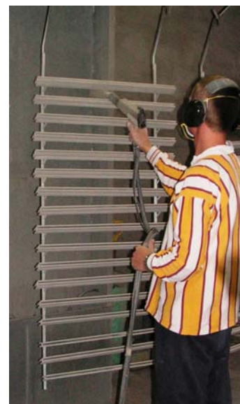
Electrostatic spray painting of furnishing parts
