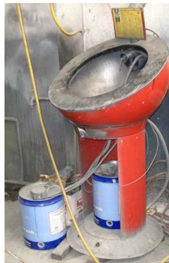
Carefully designed equipment for clean-up and disposal of thinners and cleaning solvents can reduce solvent emissions
